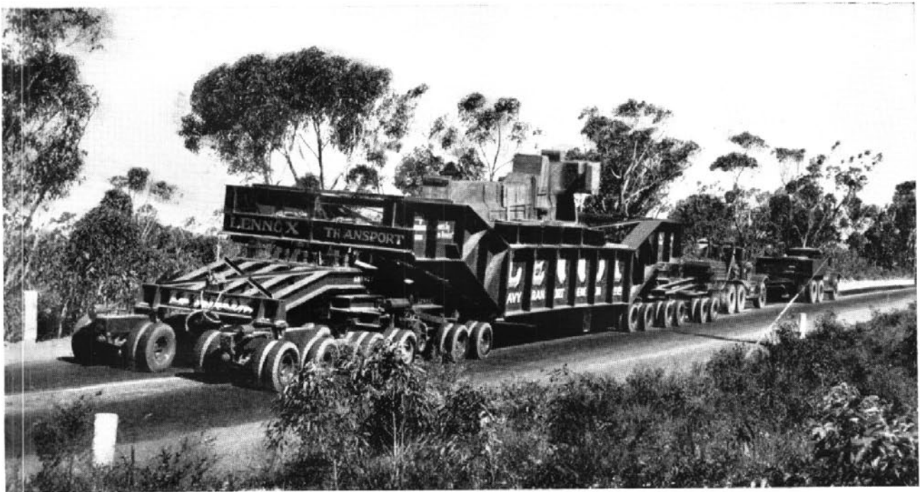
Vehicle and load having combined weight of 200 tons in transit between Walsh Bay, Sydney, and Port Kembla.
