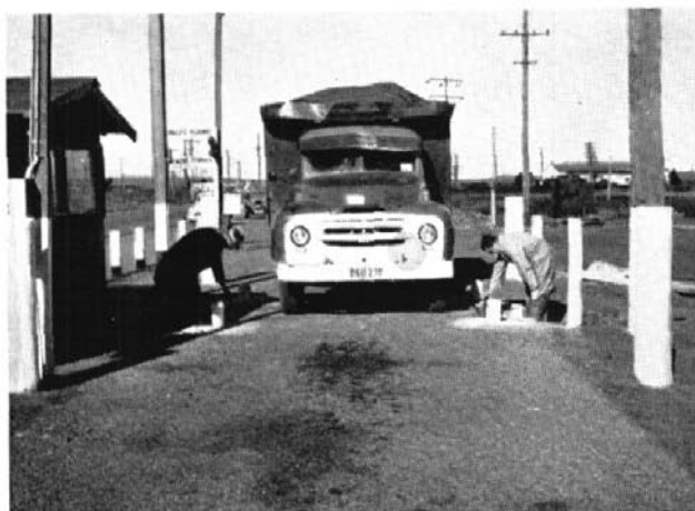
Loadometer weighing station operated by Department of Main Roads, at Hexham.
