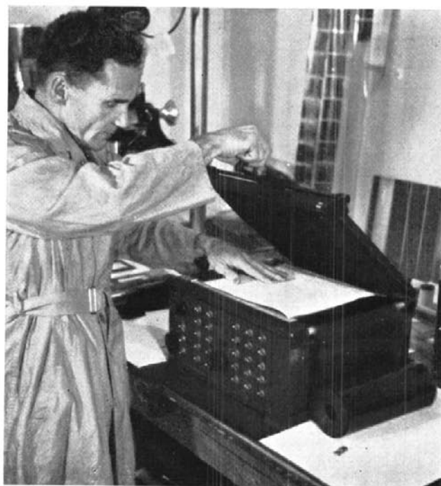
Contact printer for aerial photographs.
