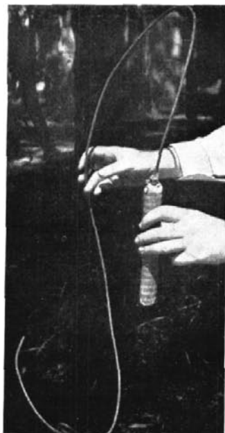
Explosive cartridge primed with plain detonator and safety fuse.
