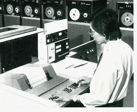
The console typewriter of the Honeywell computer is the communications link between the operator and the system.
