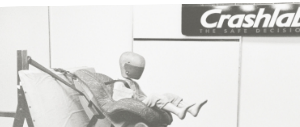
Child restraints are tested at the RTA's Crashlab
