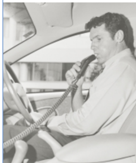
An interlock device requires the driver to pass a breath tested to enable the engine to start
