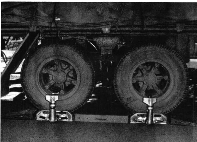
Loadometers in position
