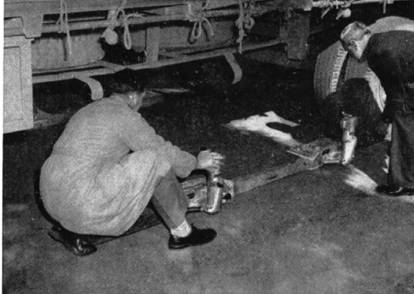
Loadometers being placed in position to weigh tandem axle load
