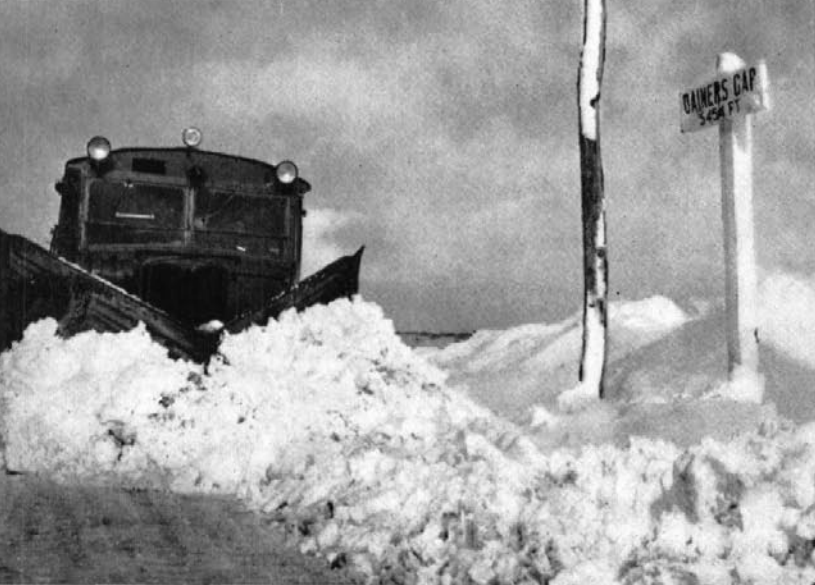
V-snow plough in operation at Dainers Gap, Mount Kosciusko Road
