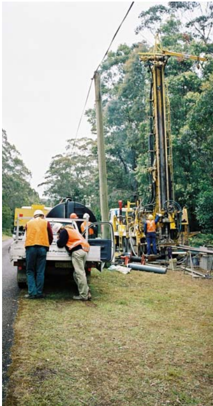
Drilling investigations to determine site conditions prior to proposed mining by Dendrobium Colliery adjacent to Cordeaux Reservoir in 2004.
