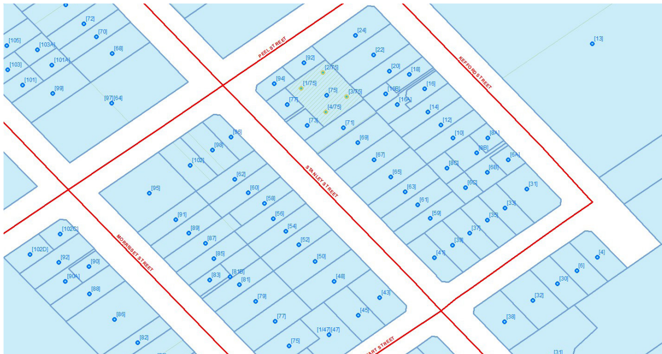
Image depicts Address Points labelled with House numbers and situated at centroid of Property. NB Building Address Points are displayed in brown colour and are situated over buildings © DFSI Spatial Services 2018
