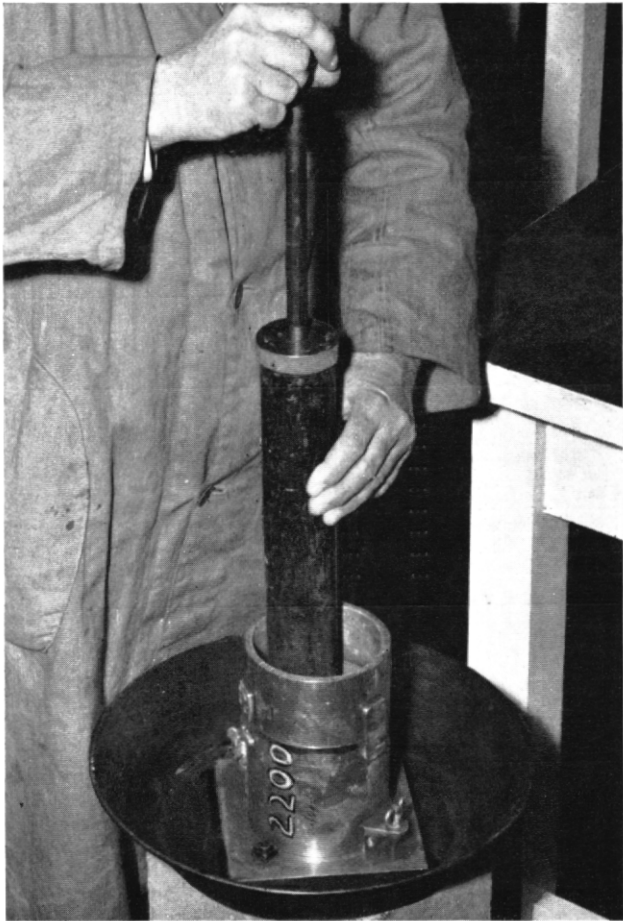
Proctor Compaction Test.—Soil being tamped in mould with standard Proctor rammer.
