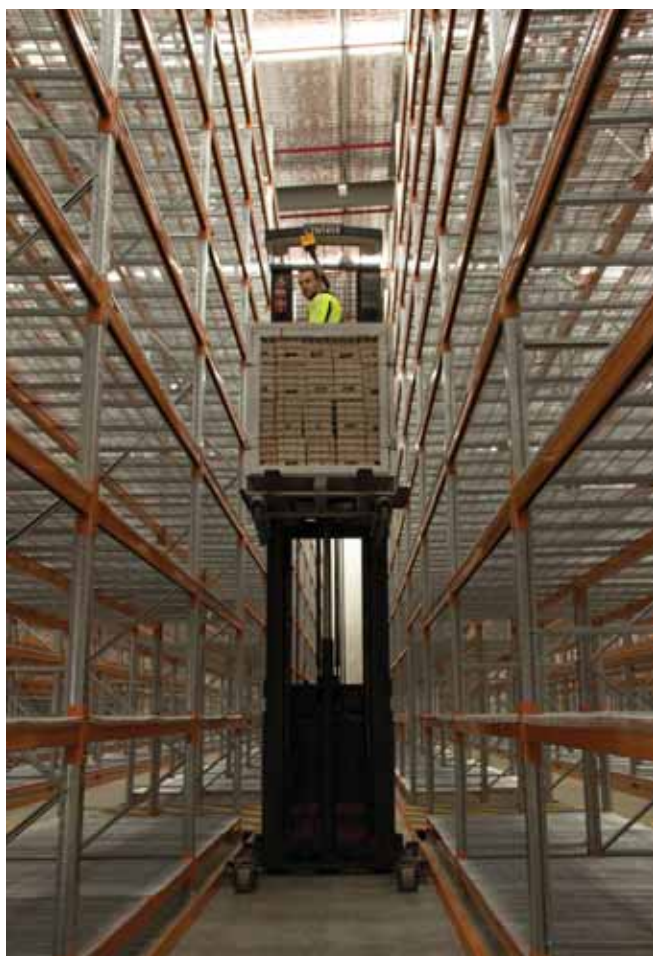
FIGURE 56: Order picker as used in the GRR off-site repositories.
