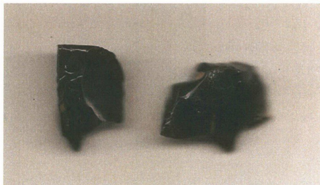
Plate 2: View showing inner and fractured surfaces of glass
